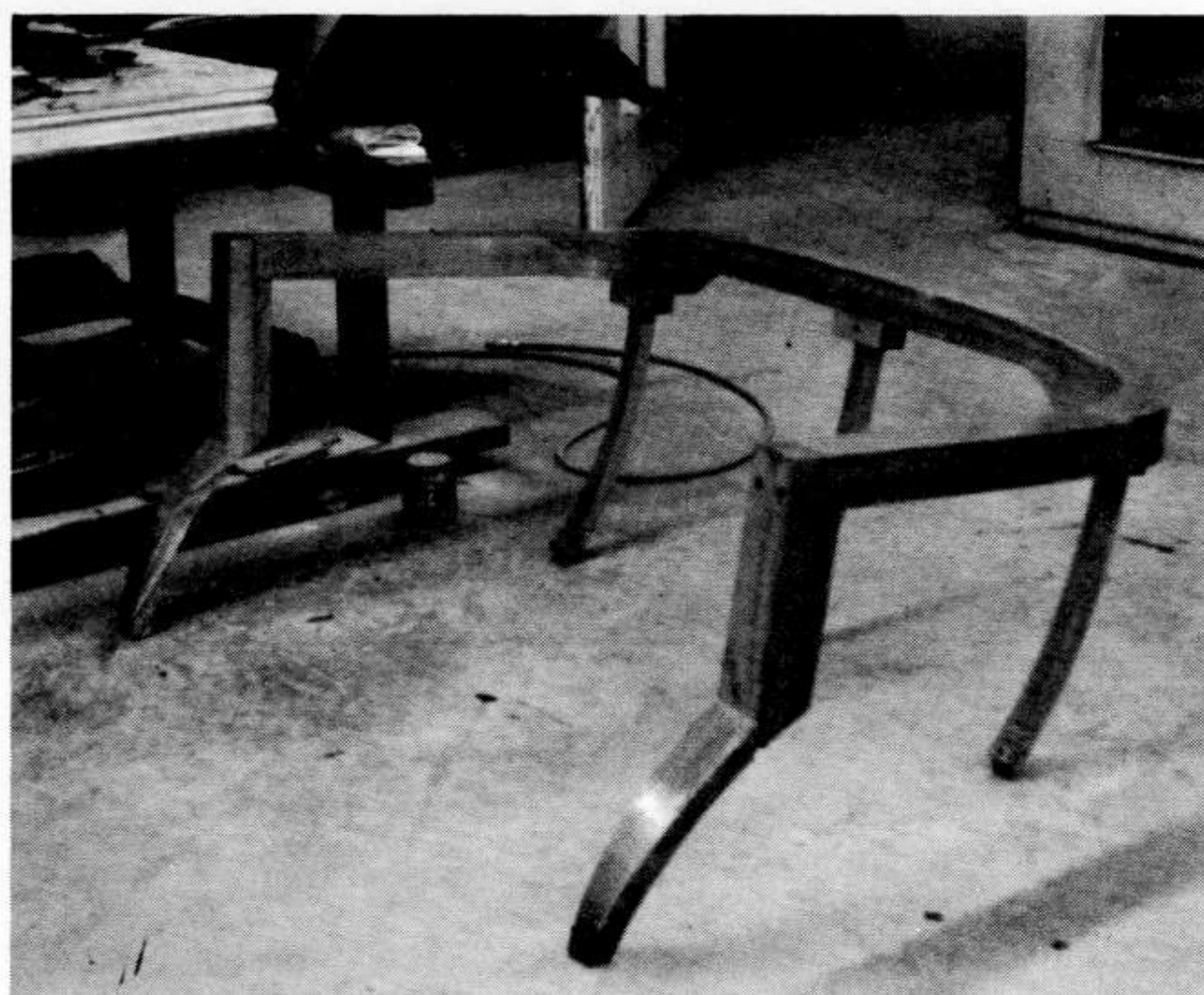
All new wooden body framing was required.
