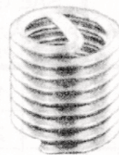
A Heli-Coil® - a 'new' thread - is screwed into an enlarged threaded hole. The crossbar shown in the illustration is broken off after installation.
