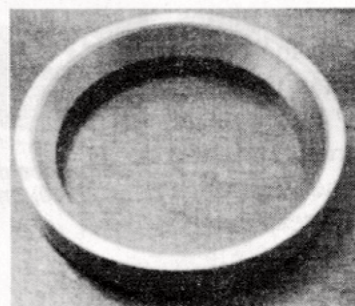
A hardened exhaust valve seat is highly recommended with unleaded gasoline.
