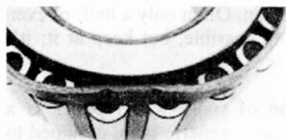
Above: a damaged bearing cage.
