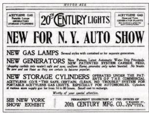
Figure 7. Advertisement from a January 1905 issue of Motor Age. This is a very early mention of dissolved acetylene for automobile use and shows the minimum duration of 14 hours based upon the maximum draw rate of seven percent of the nominal volume per hour.
