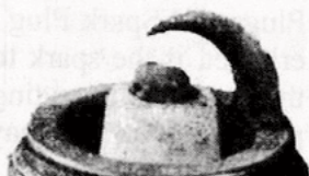
The severely worn ground electrode is evidence of a long, hard life. Replace the plug.
