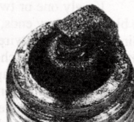
Oily Buildup of Sludge
