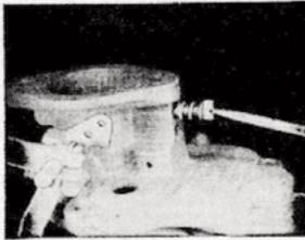
**28. Install idle adjustment screw and spring.**
