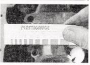
Match the width of the stripe against the calibrated gauge card supplied and read off the clearance.
