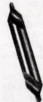
A starter bit is designed specifically for starting a pilot hole.
