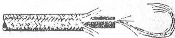
This is what most old-time auto wires look like as they're removed from the car.
