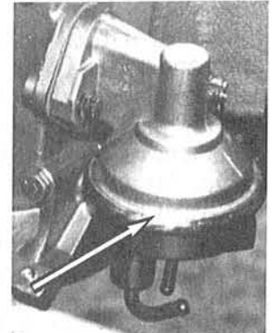
The top of the fuel pump is crimped onto the lower section. It was not designed to be rebuilt.
