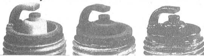
Left: a normal spark plug in good condition. Tip is a dry, light tan color. Center: Too rich a fuel mixture. Tip is a dry, chalky black color. Right: An oil leak in valves or rings. Tip is an oily wet black.
