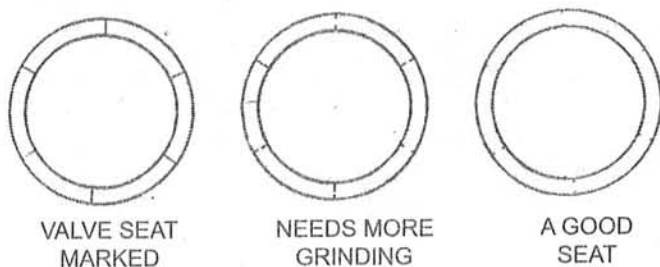
TESTING THE VALVE When all pencil marks or chalk marks are rubbed out throughout the greater part of their length, a good gas-tight seat has been achieved.
