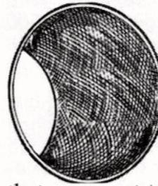
*A cross-hatch pattern on the cylinder wall will help the new rings seat to the bore. If the cross-hatch is in good condition when the cylinder is cleaned, honing may not be necessary. If the cylinder has to be honed, a minimum of honing should be done - just enough so that the cross-hatch pattern is distinct.*
