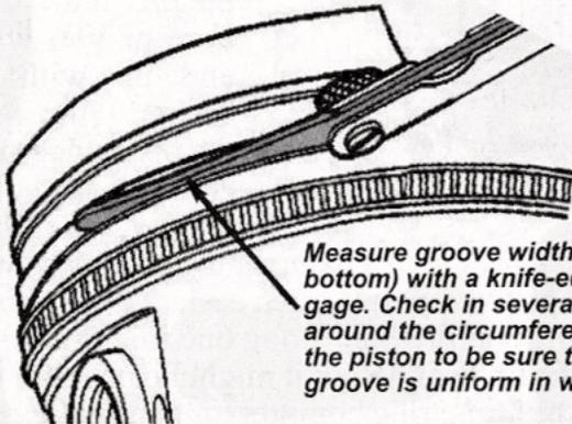
Measure groove width (top-to-bottom) with a knife-edge feeler gage. Check in several spots around the circumference of the piston to be sure that the groove is uniform in width,
