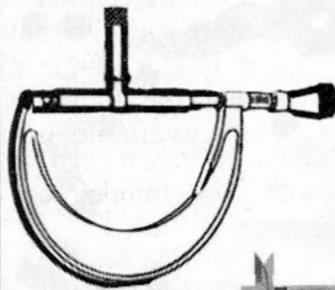
The bore should be measured with a telescoping gage (gage lengths are available in sets to fit a variety of bore sizes). Measurement should be taken in several places and in several positions within the bore
