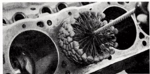
more than one minute per bore (that a maximum of 30 up and 30 down motions).
