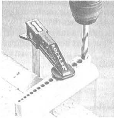
A drill guide will help keep a hand drill perpendicular to the work piece.
