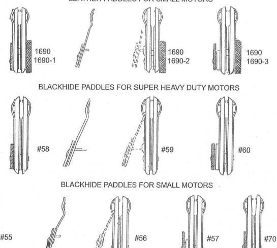
The most essential individual part in the assembly of a windshield wiper is the part which Trico terms "the paddle".
