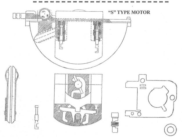
In the "S" type motor a piston type valve action is used. Follow the course of the air column from the hose connection across the top of the wiper and notice that this passage has two outlets which are alternately opened and closed by the up-and-down action of the valve stems. The valve stems themselves are operated up and down by means of the valve mechanism illus-
